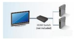
**Note:** If not connecting a repeater, the maximum length of HDMI cable allowed is 15m. To reach a longer distance, please use CAT6 cable or a repeater. HDMI converter is used to detect the monitor and correctly output.
